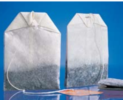
High-quality abaca ("Manila hemp"), cellulose fibers and man-made fibers form the basis of these papers. For heat sealable teabag filter papers, a special sealing layer of polyethylene, polypropylene or copolymers is added.
