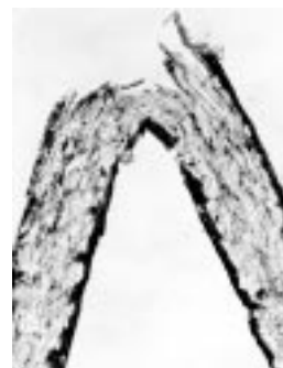
Figure 7. Fold cracking may occur when the paper is too dry. The moisture content of the sample in the center example was 20% RH; that on the right 50% RH.
