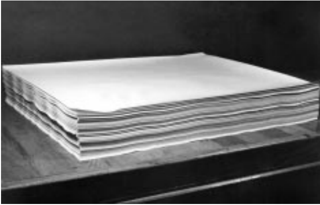
Figure 6. “Wavy” edges and “tight” edges are caused when the edges of the paper expand or contract relative to the middle of the sheet.
